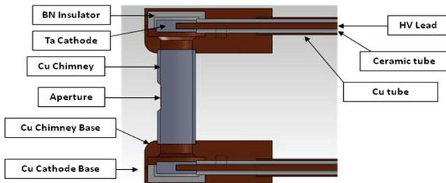
Figure 2: Cross sectional view of the PIG source.
