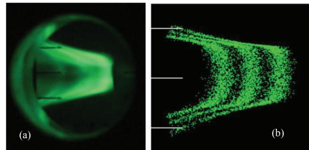
Figure 8: (a) Beam transported through the deflection channel and onto a phosphor screen, (b) SIMION simulation of the observed  $n$ ,  $n+1$ ,  $n+2$  turns.
