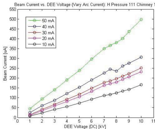
Figure 3: DC Characterization of proton beam current for a 1/32 inch diameter aperture for several arc currents.
