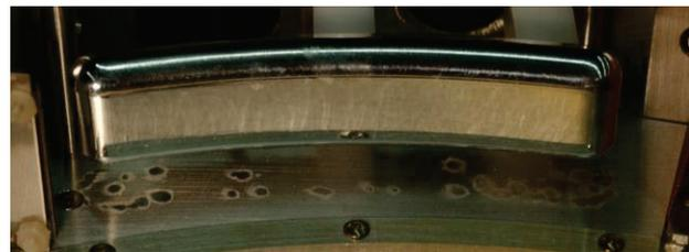
Figure 6: Partially disassembled deflector revealing pitting on bottom (and top) lids from internal arcing.
