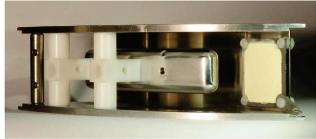
Figure 5: Electrostatic deflector assembly.
