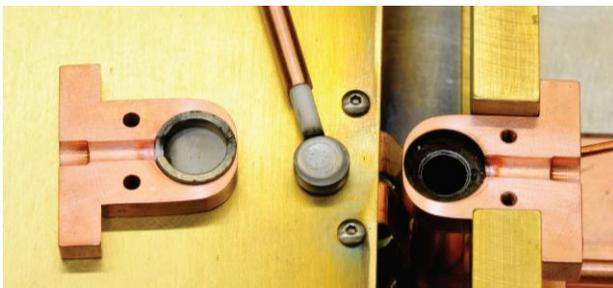
Figure 4: Source disassembled showing erosion and buildup of Ta in the BN cup and chimney base.
