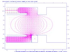
Fix.5 PSF model showing suppression of e-.
