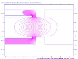
Fig. 3 PSF model of DEE-Dummy DEE
