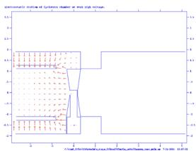
Fig.6 Plot of E-field vectors near ion aperture.
