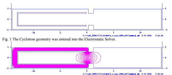
Fig. 2 Superfish's Electrostatic Solver's output, displaying lines of constant potential.
