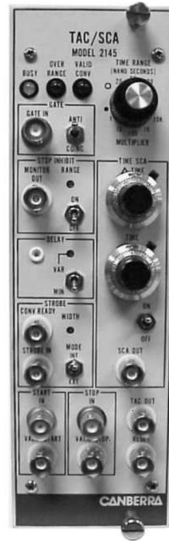
Following a valid conversion, the STROBE function allows an external control signal to determine if and when a TAC output is generated. The start and duration set the time window during which a strobe signal will be accepted. They are controlled by the DELAY and CONV READY signals respectively. In the EXT STROBE Mode, the DELAY and CONV READY signals allow minimization of system dead time.
