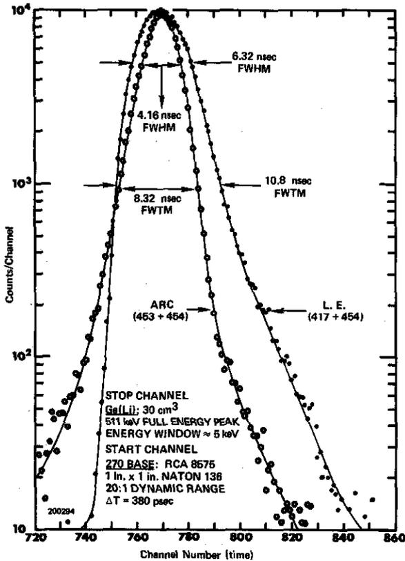
Fig. 7.2. Ge(Li) Leading Edge vs ARC Timing.
