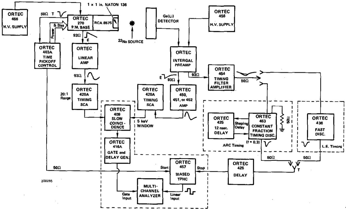
Fig. 7.1. Block Diagram Showing Leading Edge (L.E.) Timing vs Amplitude and Risetime Compensated (ARC) Timing Systems for Ge(Li) Detectors.
