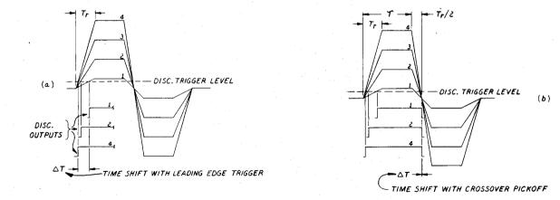
Figure 1. Timing From Linear Amplifier Output Pulses
