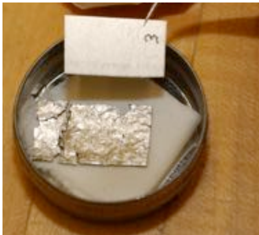
Figure 5. Comparison of two initially identical titanium samples. Swelling and embrittlement of the loaded sample is pronounced.
