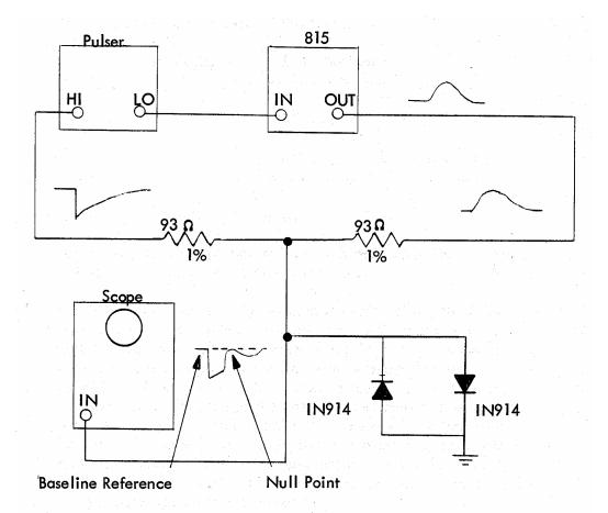
Adjust pulser output so high output is nearly 10 volts; adjust amplifier gain so its output is nearly 10 volts; observe difference on oscilloscope using test circuit; adjust amplifier Fine Gain so null point is at baseline reference level. The linearity of the amplifier may now be tested by increasing the oscilloscope sensitivity to maximum, adjusting the Model 815 Fine Gain to reposition the null point at baseline reference, and then turning the pulser output from maximum down to zero.
